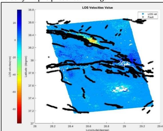
**Figure 4.** Sentinel 1A 131 frame Ascending LOS significant velocities
