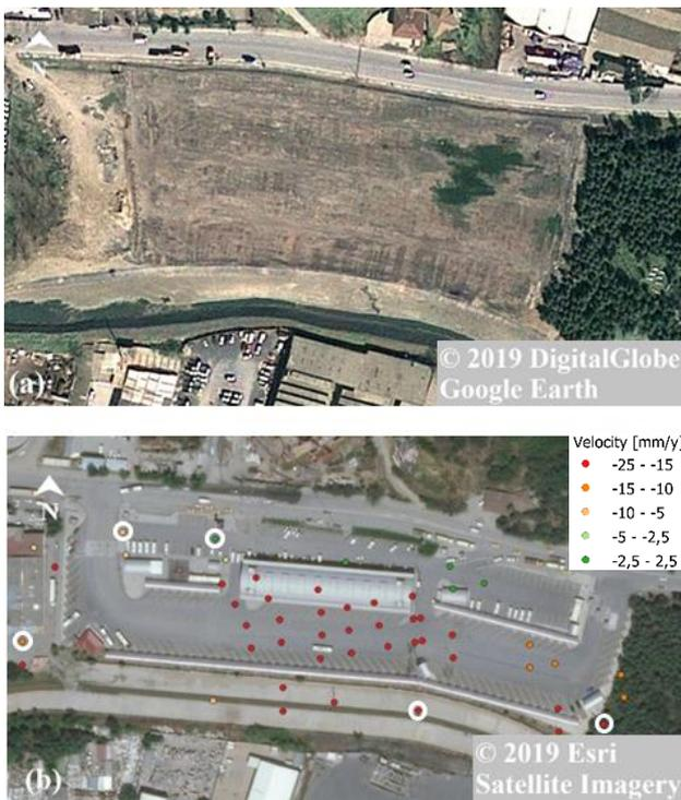
Figure 5. (a) Optical image of Alibeykoy Mobile Bus Station 2011. (b) Same view in 2019, with overlying PSs representing the average 2015-2018 velocity measurements of displacement in mm/years.
