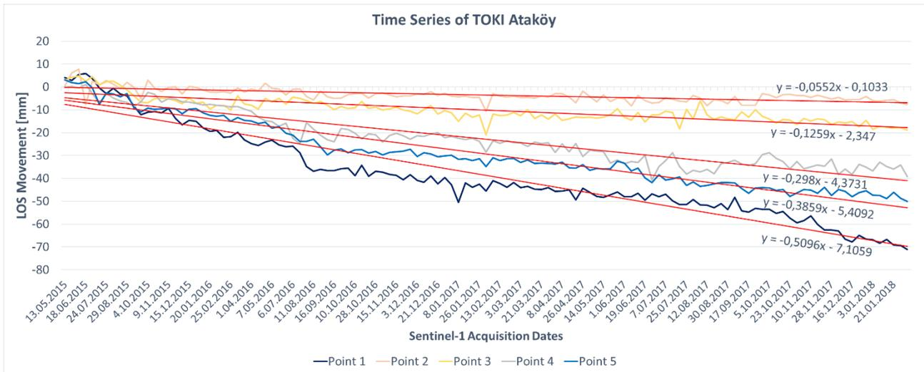
Figure 4. Movement of five PSs attributed to the Atakoy Residential site over time. The location of the PSs can be seen in Figure 3(b) with white circles.
