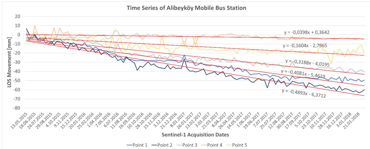
Figure 7. Movement of five PSs attributed to the Alibeykoy site over time. The location of the PSs can be seen in Figure 5(b) with white circles.
