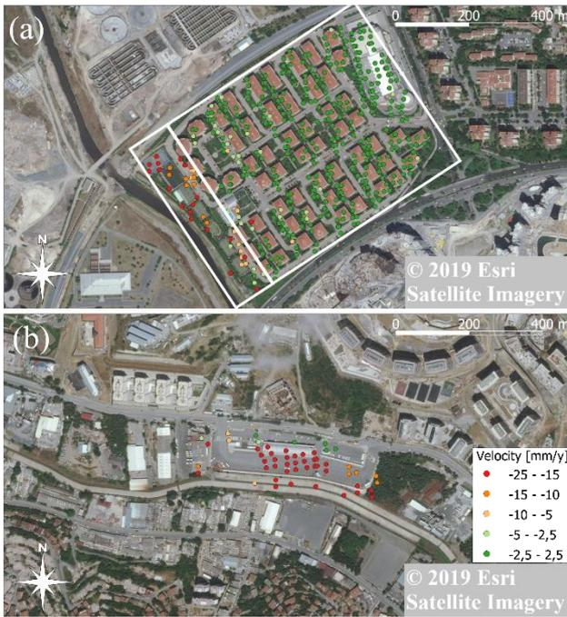
Figure 2. Persistent scatterers with their mean velocity superimposed over Google Earth images of the two test sites.
