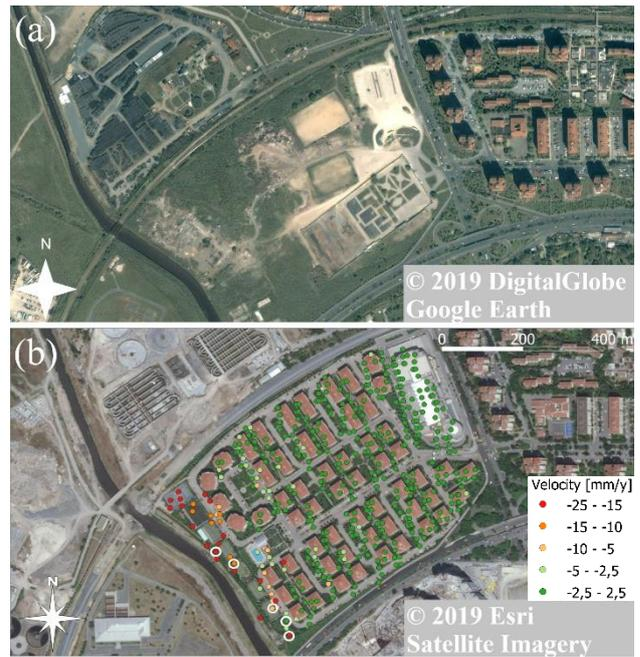
Figure 3. (a) Optical image of TOKI Atakoy residential area in 2001. (b) Same view in 2019, with overlying PSs (dots) representing the average 2015-2018 velocity measurements of displacement in mm/years. Ground subsidence is clearly visible closer to the creek.
